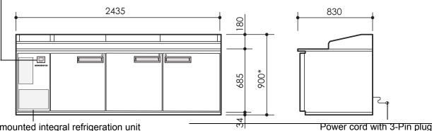
Side mounted integral refrigeration unit Copyright © 2012 SKOPE Industries Limited
