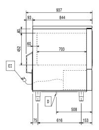
Drain Electrical inlet (power)
